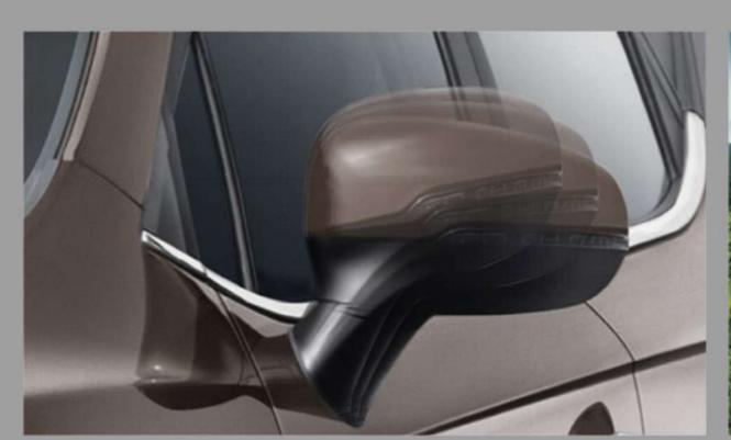
Automatic side mirrors- the rearview mirror will automatically fold when locked avoiding unnecessary collision
